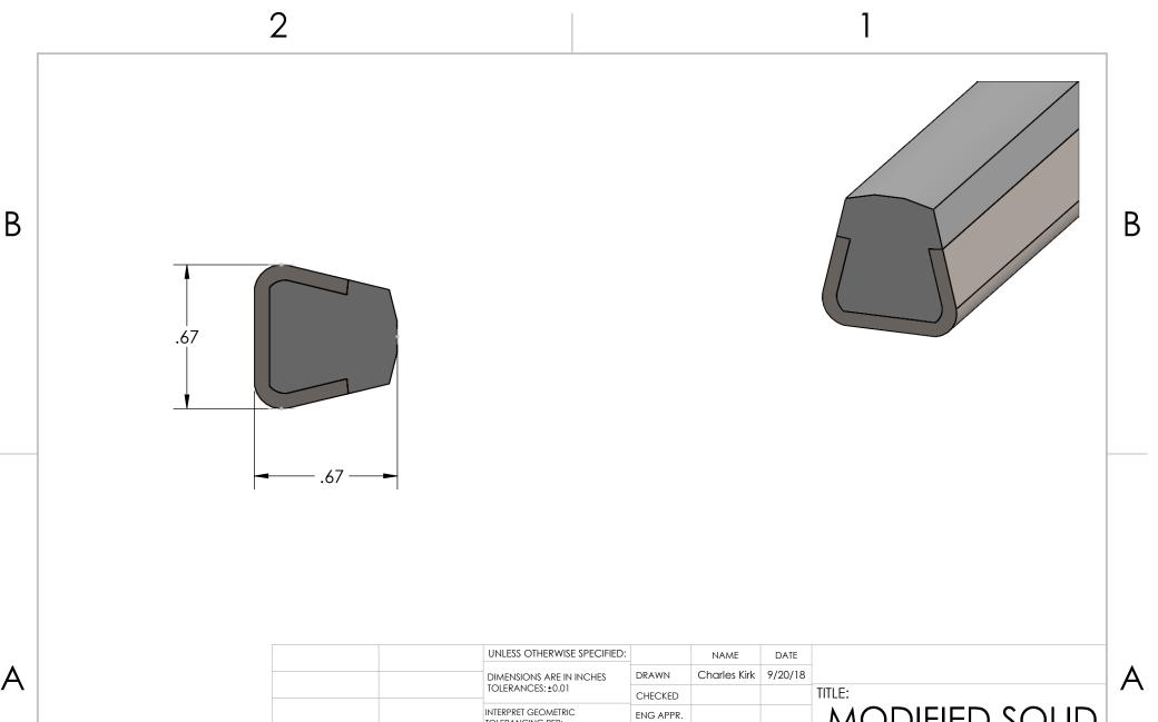
MODIFIED SOLID TOLERANCING PER: MFG APPR. **GUIDE RAIL** MATERIAL Q.A. Natural UHMW-PE/ PROPRIETARY AND CONFIDENTIAL COMMENTS: 304 Stainless Steel THE INFORMATION CONTAINED IN THIS SIZE MPSSMS20 REV DRAWING IS THE SOLE PROPERTY OF MASON PLASTICS COMPANY. ANY FINISH REPRODUCTION IN PART OR AS A WHOLE NEXT ASSY **USED ON** 2B WITHOUT THE WRITTEN PERMISSION OF MASON PLASTICS COMPANY IS SCALE: 1:8 WEIGHT: SHEET 1 OF 1 PROHIBITED. APPLICATION DO NOT SCALE DRAWING
