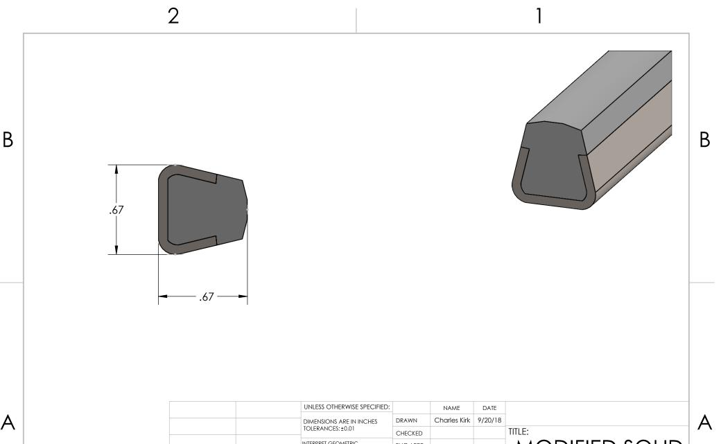
MODIFIED SOLID INTERPRET GEOMETRIC ENG APPR. TOLERANCING PER: MFG APPR. **GUIDE RAIL** MATERIAL Q.A. Natural UHMW-PE/ PROPRIETARY AND CONFIDENTIAL COMMENTS: 304 Stainless Steel THE INFORMATION CONTAINED IN THIS SIZE MPSSMS05 REV DRAWING IS THE SOLE PROPERTY OF MASON PLASTICS COMPANY. ANY FINISH REPRODUCTION IN PART OR AS A WHOLE NEXT ASSY **USED ON** 2B WITHOUT THE WRITTEN PERMISSION OF MASON PLASTICS COMPANY IS SCALE: 1:8 WEIGHT: SHEET 1 OF 1 PROHIBITED. APPLICATION DO NOT SCALE DRAWING
