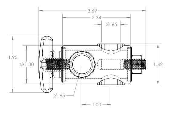
UNLESS OTHERWISE SPECIFIED: NAME DATE Charles Kirk 12/10/18 DRAWN DIMENSIONS ARE IN INCHES TOLERANCES: ±0.01 CHECKED Cross Block for ENG APPR. MFG APPR. 5/8"x5/8" Rods INTERPRET GEOMETRIC Q.A. PROPRIETARY AND CONFIDENTIAL TOLERANCING PER: COMMENTS: THE INFORMATION CONTAINED IN THIS MATERIAL SIZE DWG. NO. DRAWING IS THE SOLE PROPERTY OF MASON PLASTICS COMPANY. ANY FINISH
