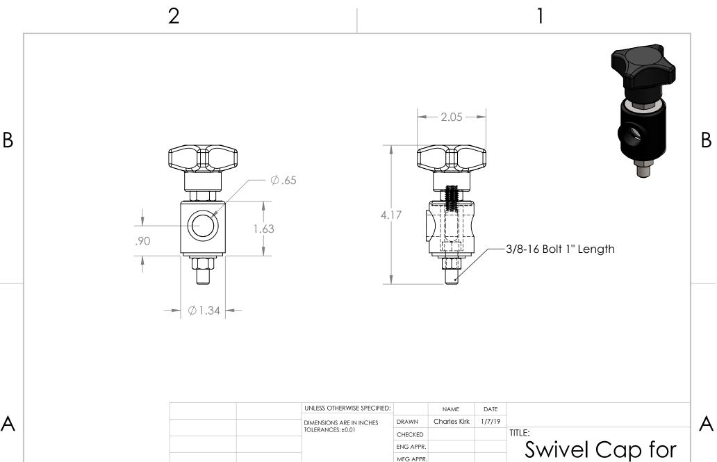
Swivel Cap for 5/8" Rods MFG APPR. INTERPRET GEOMETRIC Q.A. PROPRIETARY AND CONFIDENTIAL TOLERANCING PER: COMMENTS: THE INFORMATION CONTAINED IN THIS MATERIAL SIZE DWG. NO. REV DRAWING IS THE SOLE PROPERTY OF MP503SC58 MASON PLASTICS COMPANY, ANY FINISH REPRODUCTION IN PART OR AS A WHOLE NEXT ASSY **USED ON** WITHOUT THE WRITTEN PERMISSION OF MASON PLASTICS COMPANY IS SCALE: 1:2 WEIGHT: SHEET 1 OF 1 PROHIBITED. APPLICATION DO NOT SCALE DRAWING
